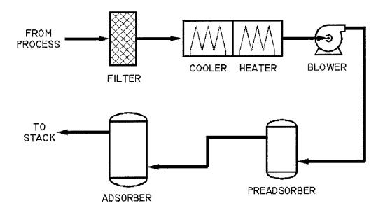
**Figure 1 Adsorption Process**
