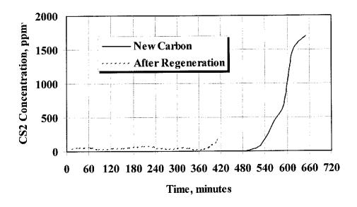
With new carbon, the time to breakthrough was just over 8 hours. After regeneration, it was reduced to just less than 7 hours. This is an indication that the regeneration was very effective. At the time of breakthrough after regeneration, the carbon had retained 12.5 g carbon disulfide /100 g activated carbon (working capacity).
